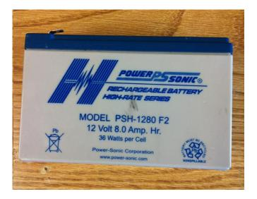
$$Battery \ Life = \frac{Capacity}{Current \ Draw} = \frac{8000 \ mA \ Hrs}{720 \ mA} \approx 11 \ Hrs$$
