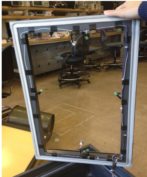
Figure E.3. Wiring of FSR, PIR and LED under the lid
