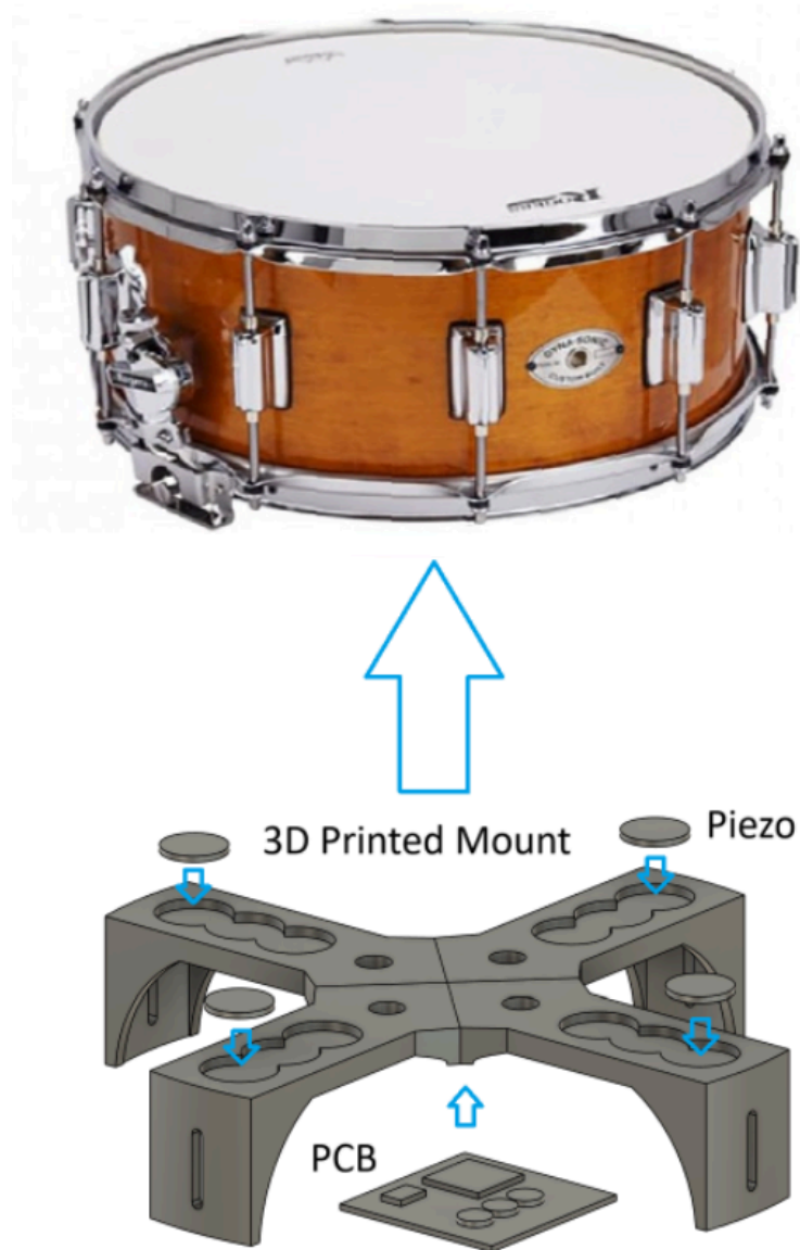
Figure 3. Physical arrangement of the drum and mounting structure with adjustable sensor mounts. Current implementation of piezo mounting and PCB mounting may be different from the realized mount.
