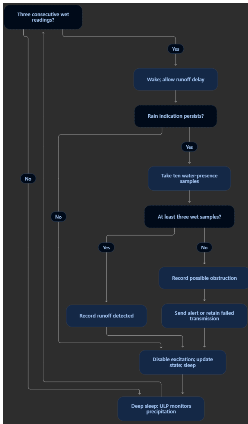
Figure 3. Proposed firmware sequence. A runoff delay precedes water-presence evaluation, and retained event state limits repeated wakeups and duplicate alerts.
