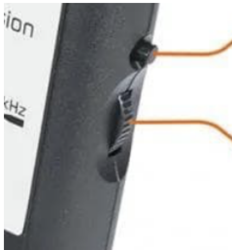
Figure 6. Volume Dial Embedded in the Housing
