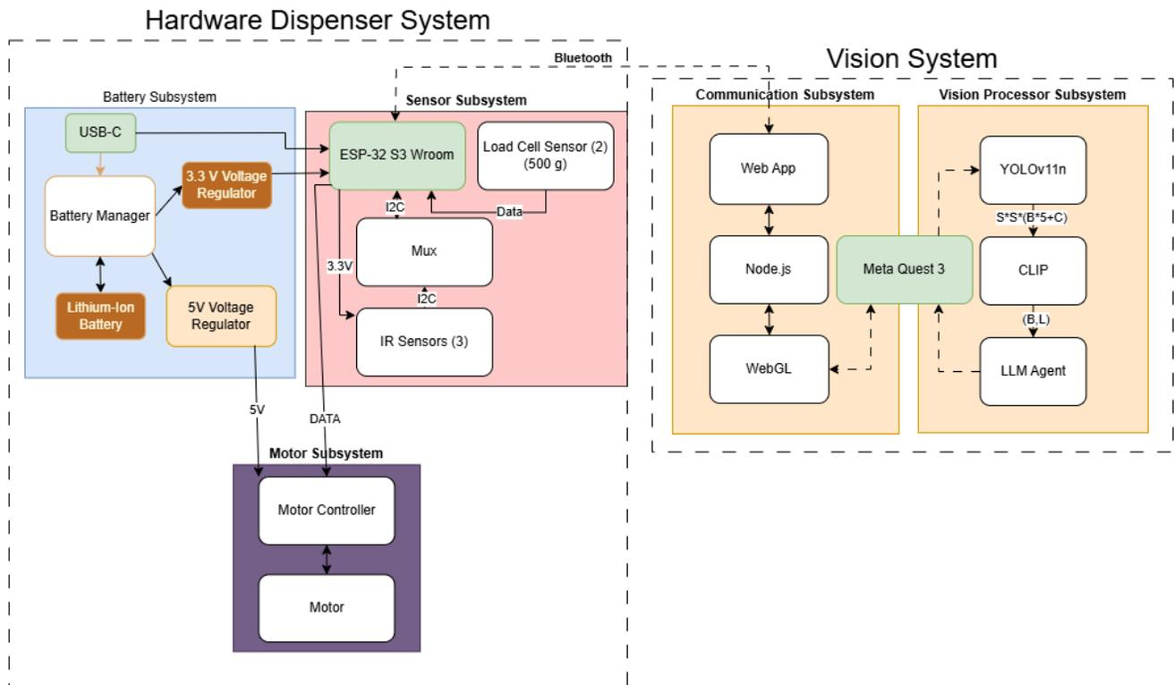
Figure 2: High-Level block diagram of the system
