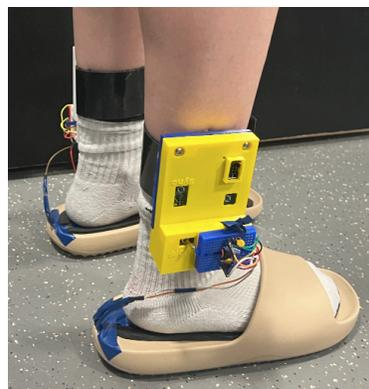
Figure 12: Final Device Assembly on User
