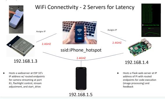
To minimize latency and ensure robust communication between modules, the system uses a shared 2.4GHz hotspot (tethered from a mobile device) to host both the ESP32-CAM and the Raspberry Pi on the same local network. Each device is automatically assigned a static IP by the hotspot's internal DHCP service. The ESP32-CAM typically receives the IP address 192.168.1.3, while the Raspberry Pi is assigned 192.168.1.4, and the mobile phone controlling the system operates on 192.168.1.5.
