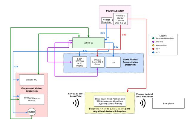
The diagram above illustrates the full system integration of our driver fatigue and alcohol detection platform, including power delivery, sensor interfacing, and wireless communication. At the core of the system is the ESP32-S3, which manages real-time data acquisition, local feedback, and WiFi communication with external processing units. The system is powered via a regulated 5V USB connection from the vehicle's console, which is stepped down to 3.3V for sensor and module compatibility.
