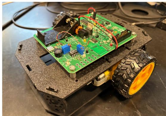
Figure 17 (above): The final PCB design fastened with spacers on the vehicle chassis.
