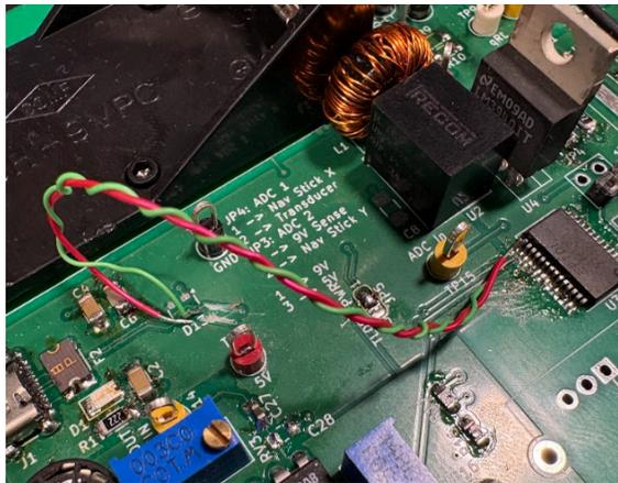
Figure 21: Bodge of the USB D+ and D- and corrected connection to the FT232RL USB to UART transceiver. [13]
