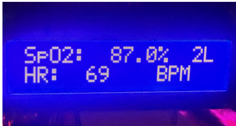
Figure 23: Layout of the Display Subsystem, SpO 2 value (top left), Mode (top right), and Heart Rate (bottom left)
