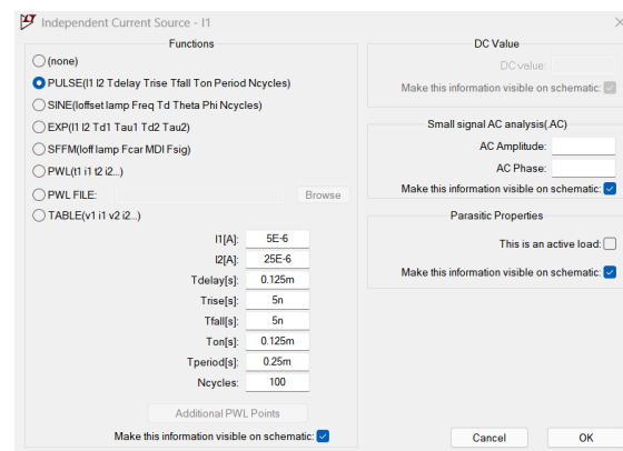
Fig. 8: LTSpice simulation square wave parameters
