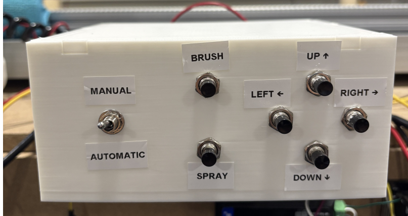
Figure 4: User interface implementation on 3D printed case
