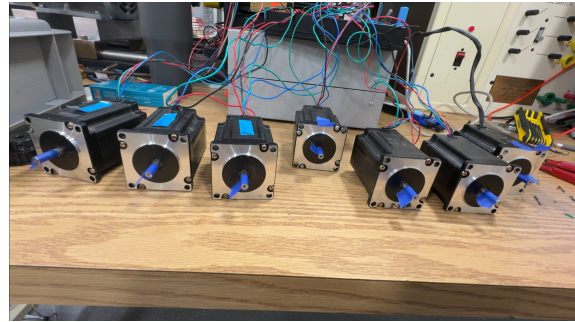
((b)) End shaft alignment at end of test
