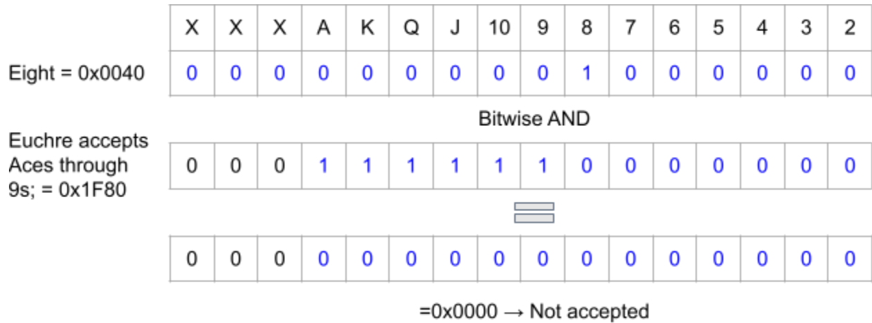
Figure 4: A diagram showing how the control system compares a card signal to the games' bitmask
