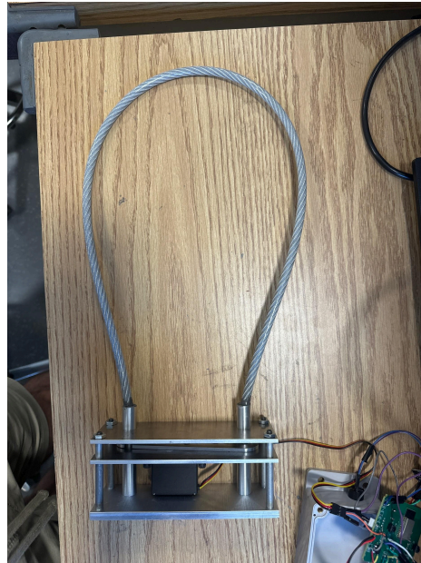
Figure 3 :Fully constructed lock with servo attached from machine shop
