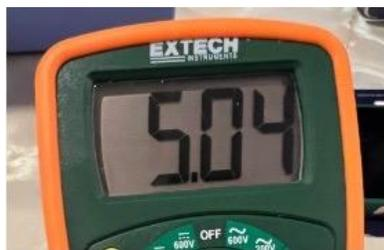
**Image 21: Camera Input Voltage**
