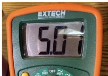
**Image 13: Proximity Sensor Input Voltage**
