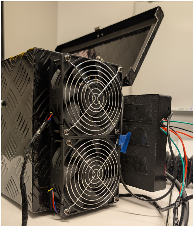
Figure 7: PWM Based Ventilation System
