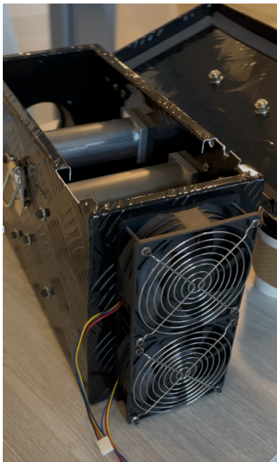
Figure 2: Fabricated Enclosure Intake
