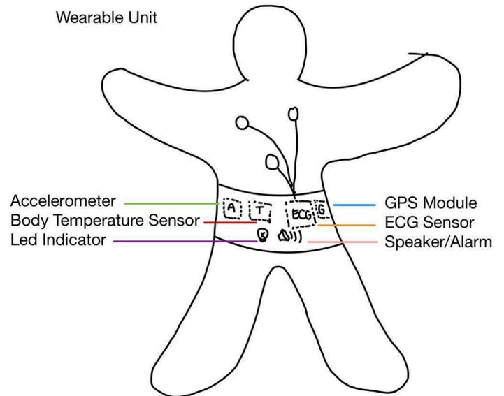
Figure 1. Design of the Monitoring Devices
