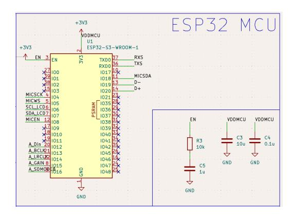
The ESP32 with Wi-Fi capability serves as the core processing unit for the entire system. It receives audio input from the microphone via the ADC, transmits the audio to the cloud-based AI model via Wi-Fi, receives the processed audio response from the AI model, and then sends the output to the audio codec for playback. This subsystem is also responsible for interfacing with the Bluetooth module for Wi-Fi configuration and managing communications with the text display for visual output.
