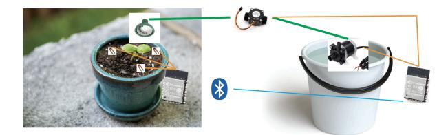
The physical design of the automated plant watering system is centered around a compact, modular setup that integrates sensors, actuators, and wireless communication. The system comprises a potted plant equipped with soil moisture sensors that are strategically embedded into the soil. These sensors continuously monitor the moisture levels and are interfaced with an ESP32 microcontroller, which serves as the central processing unit for data collection and transmission.
