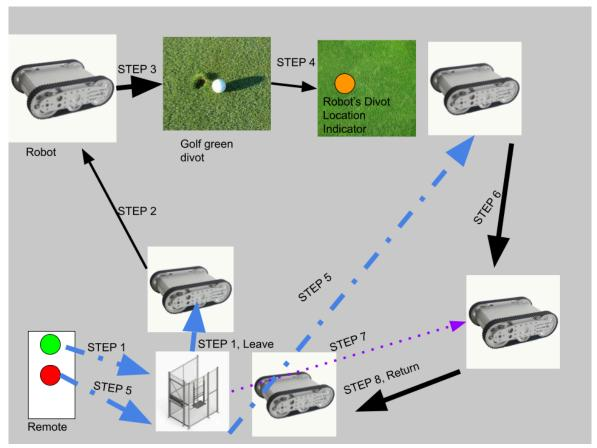
Blue arrows indicate Bluetooth Signals, Purple indicates infrared signals, black is overall traversal of the robot
