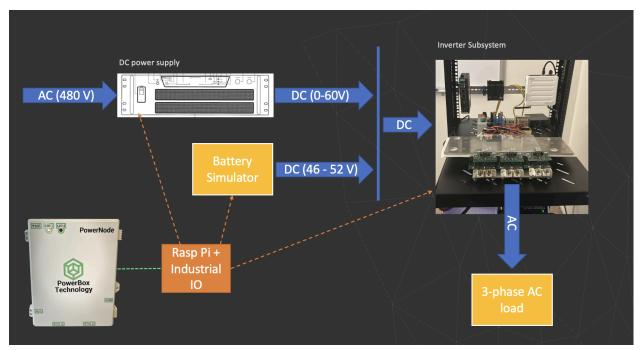
The PowerBlock includes the DC power supply, Rasp Pi + Industrial IO, inverter subsystem and our power meter. In a real setting, the battery simulator would be the battery racks shown in the picture above.
