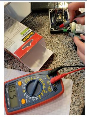
5.19V camera power voltage reading.
