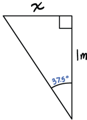
Fig. 12: Calculation of Horizontal FOV width
