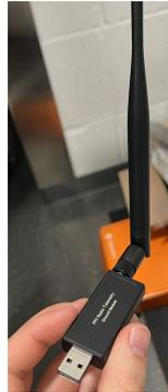
Telemetry Radio transmitter and Receiver
