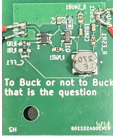
Figure 10: Physical Buck Converter
