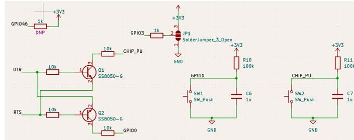
**Figure 4: ESP32 Programming Circuit**
