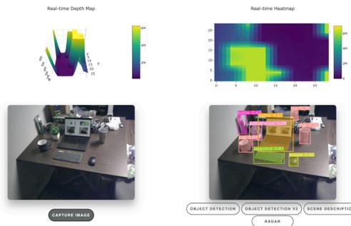
**Figure 11:** A screenshot of our web app, with imager plots (top) and object detection (bottom)
