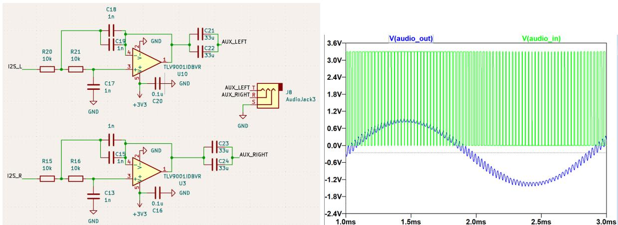
**Figure 5: Audio Subsystem Schematic simulation**
