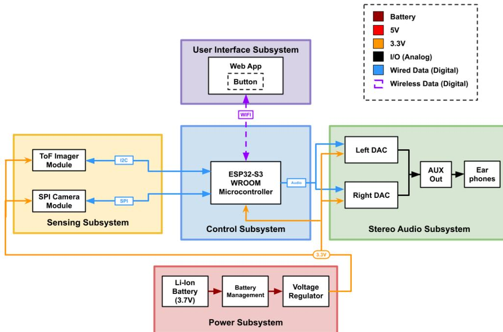
*Figure 1: Device Block Diagram*
