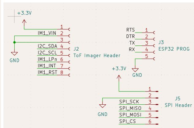
Figure 3: Input and Output headers
