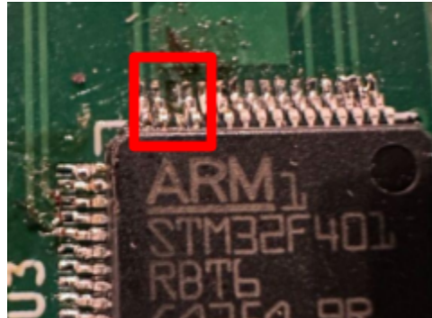
Figure 10: MCU pin broken off
