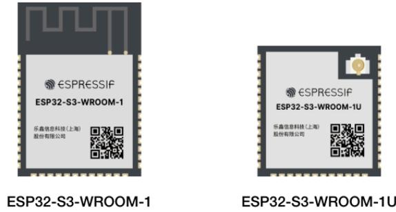
Figure 2.2.1. Top View of ESP32S3 Microchip
