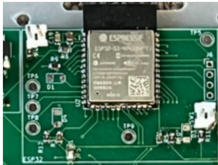
Figure 3.3 Modified PCB. Notice the white pin headers. In practice, these headers are grounded to mimic a button press.
