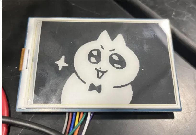
Figure 7: Digital ink screen correctly displaying the digital pet
