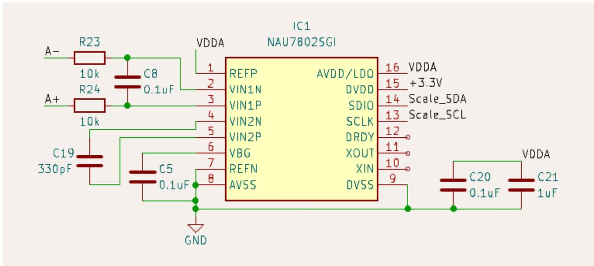
Figure 5. Load Cell ADC Converter Schematic
