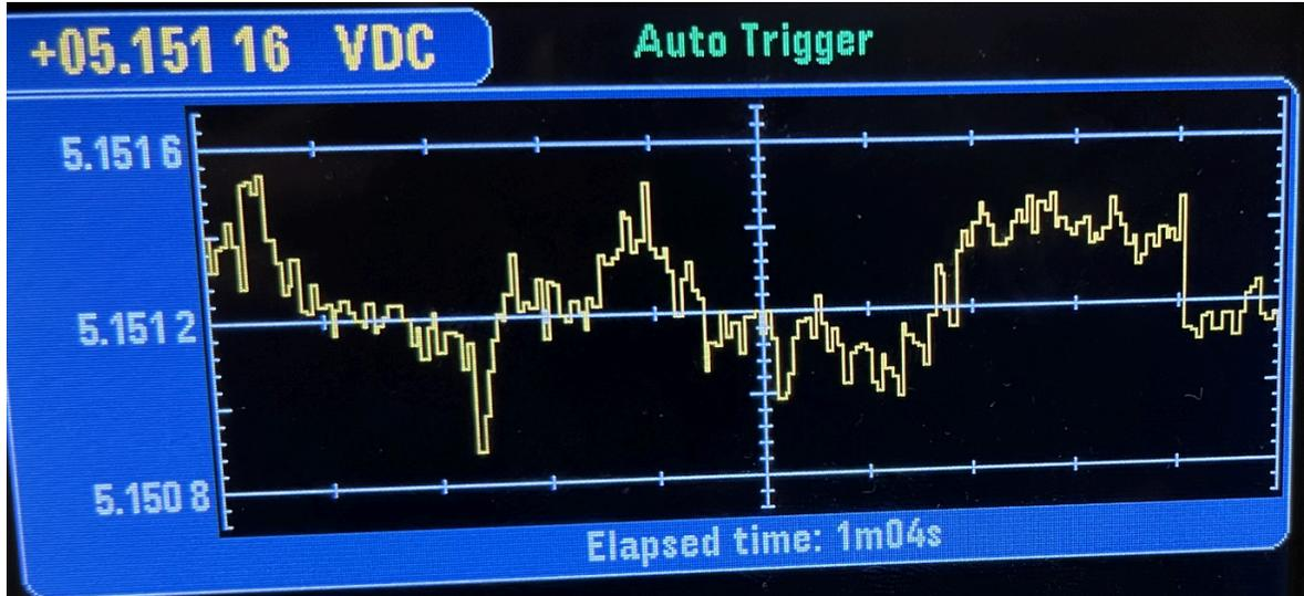
*Figure 8. 5V Scope Capture*
