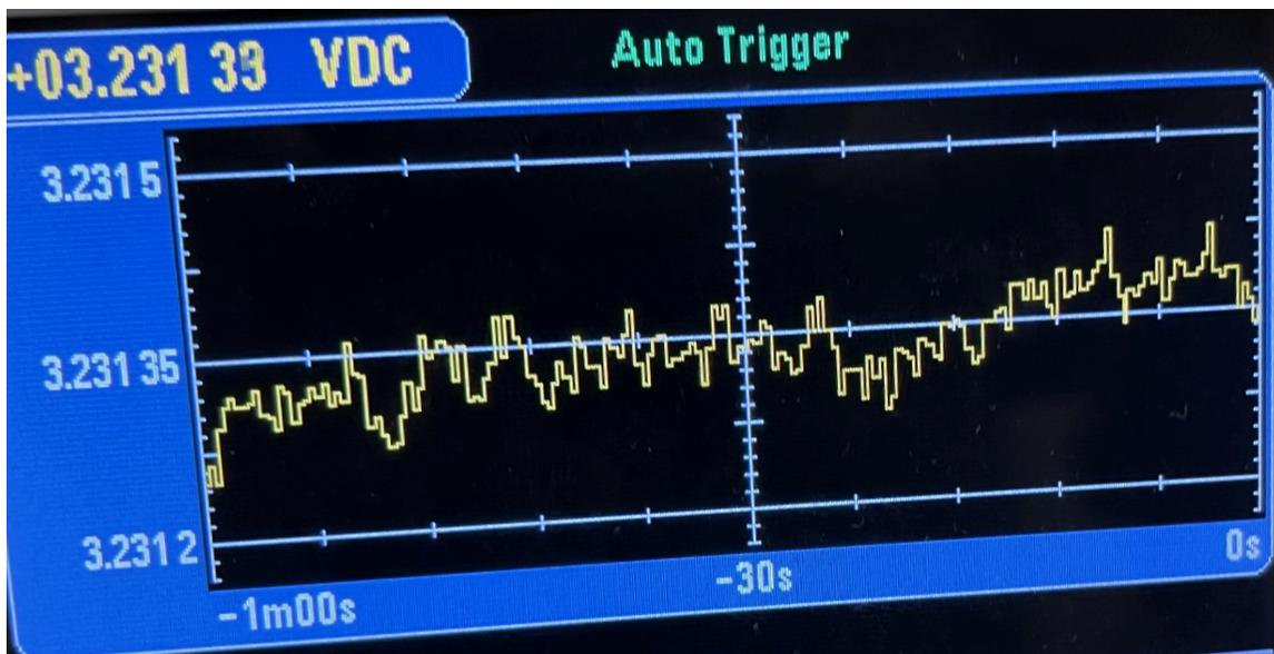
Figure 7. 3V3 Scope Capture
