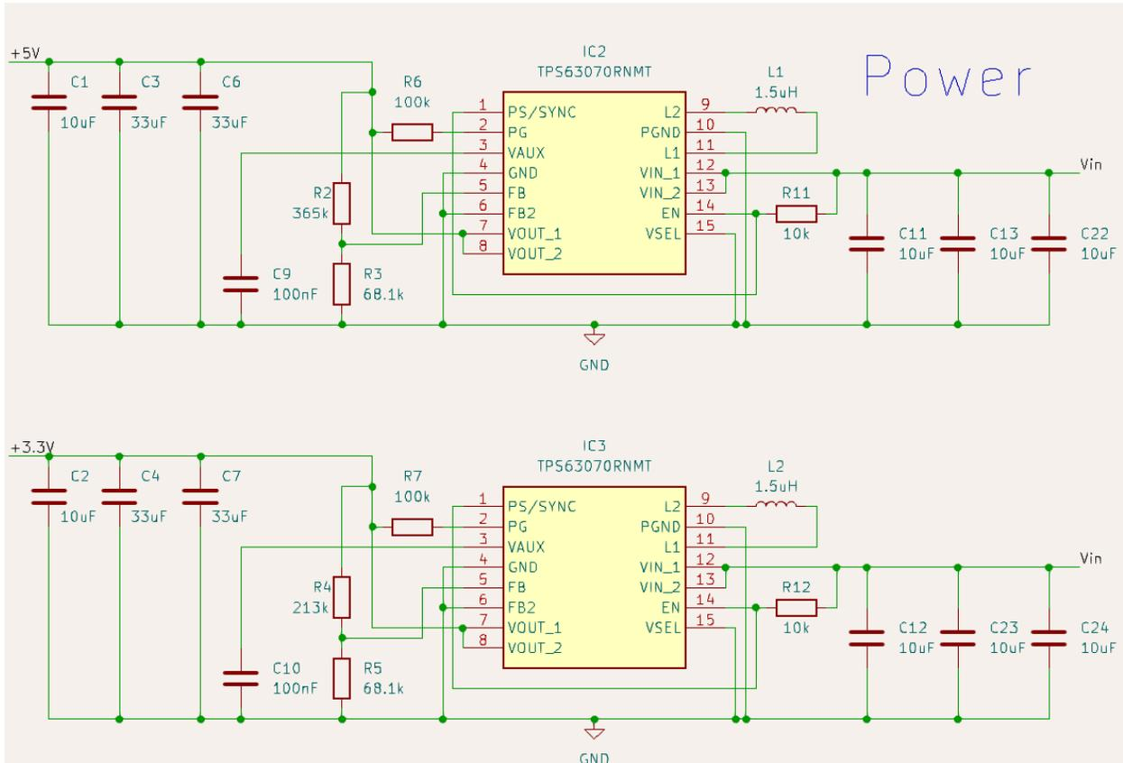
Figure 6. Buck Converter Schematics, 5V (Top) 3V3 (Bottom)
