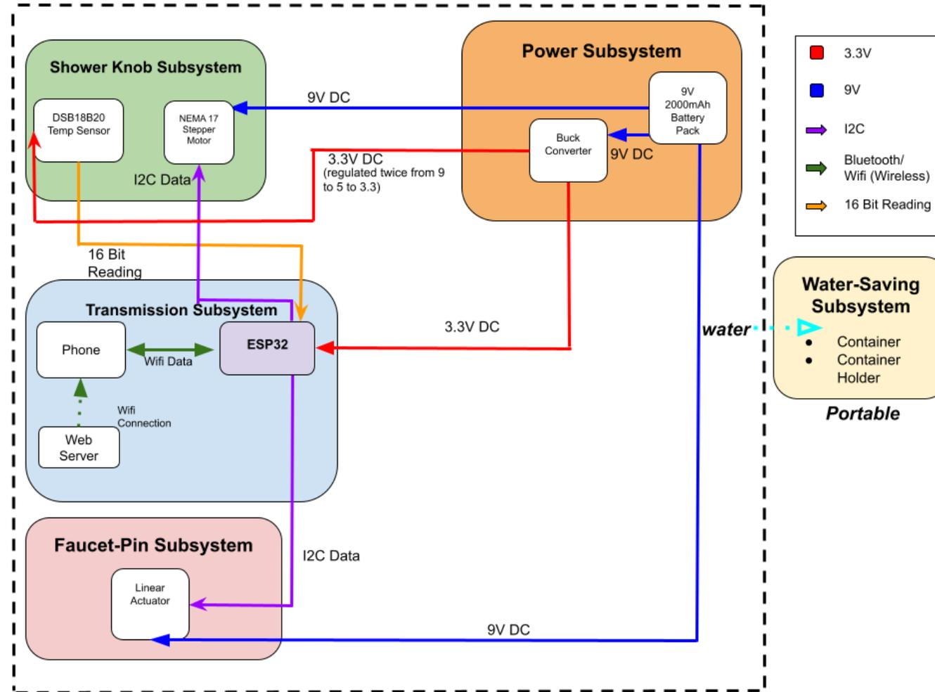
Figure 3: Overview of Each Block Requirement
