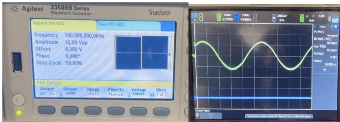
Figure 17 and 18: Figure 17(left) shows the input which is a square wave. Figure 18(right) shows the output on the receiving side – a sine wave of the same frequency
