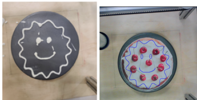
Fig.14 shape drawn by the machine(left one) shape predefined by program(right one)
