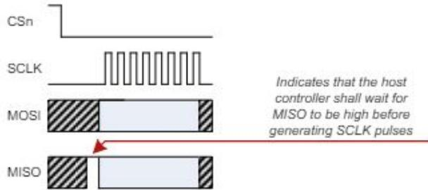
Figure 52 – SPI interface wait state
