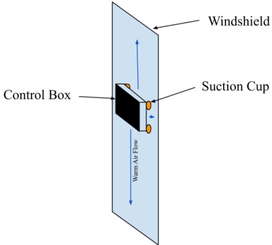
Figure 2: Visualization of how the Control Box would deliver heat.
