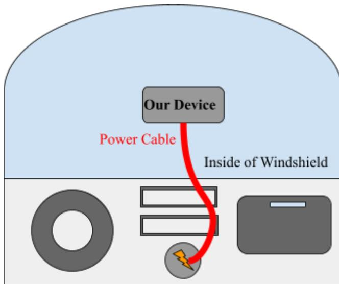
Figure 3: Visualization of how the Control Box would be attached inside the windshield.
