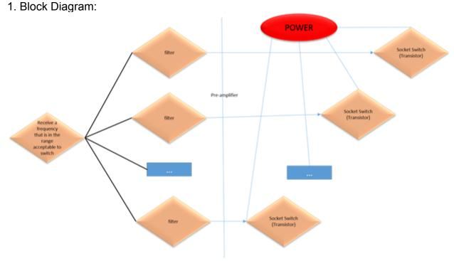
**Power**: The power block is the source from the wall.
