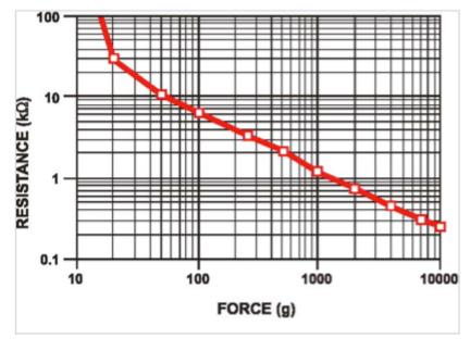
The sensing unit consists of the Model 400 Force Sensitive Resistor(FSR) that would be placed behind the LEDs on the fretboard. The FSR is 0.2" [5mm] in diameter and will register a pressure value when the user presses the desired note. We will be implementing the FSR as an on/off switch and use the breakpoint located at approximately 30,000 ohms to determine whether or not the user is applying
