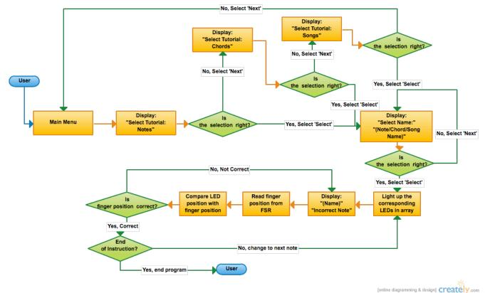
The push buttons on the LCD allow the user to select what option they prefer. They include "Select", "Up", "Right", "Down", "Left" and "Reset".
