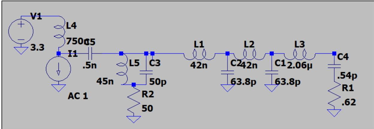
Figure 11 - Class E amplifier Matched load
