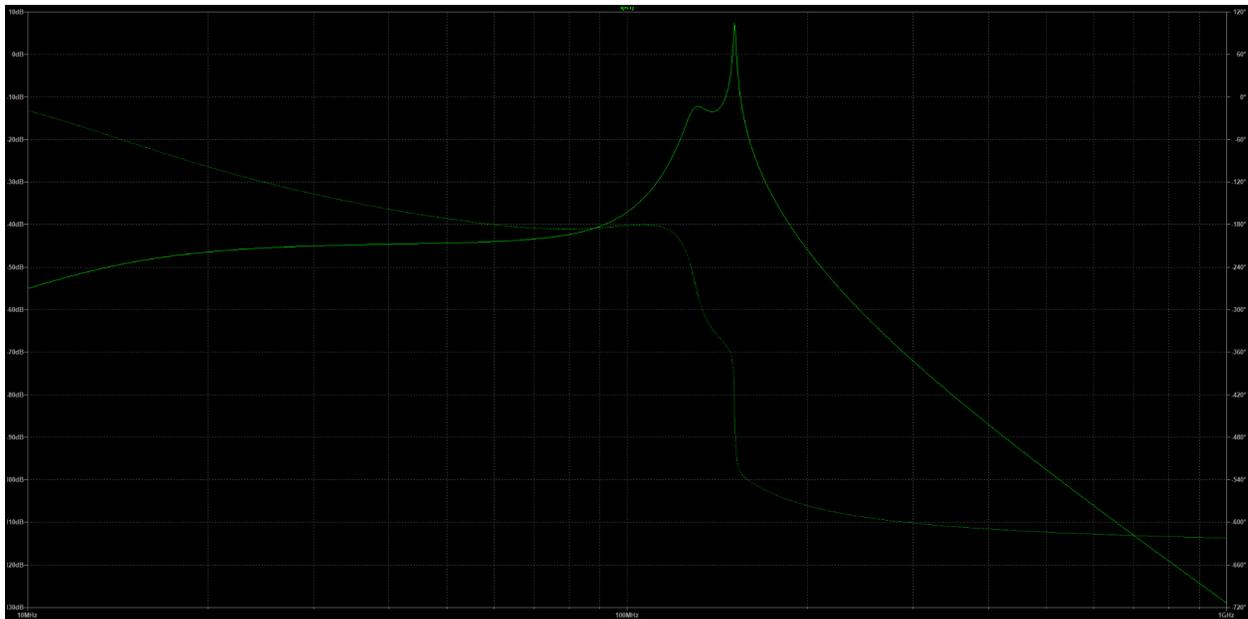
Figure 12 - Class E amplifier matched load bode plot
