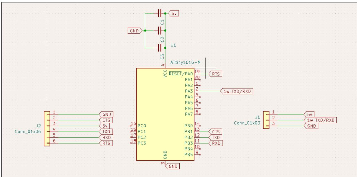
**Figure 13 - Microcontroller and control schematics**
