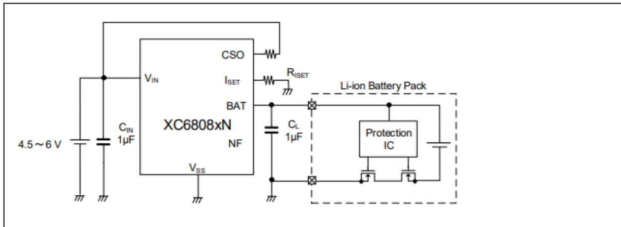
**Figure 3 - Charger Circuit**
