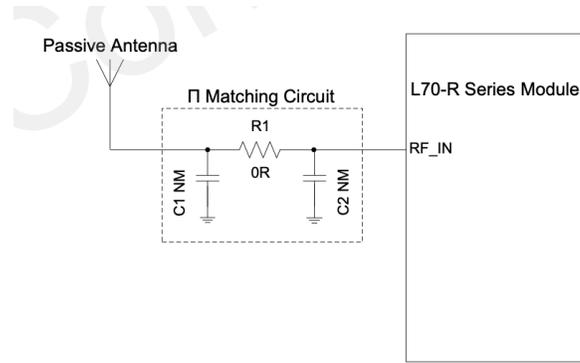
**Figure 7:** Reference Design for a Passive Antenna
