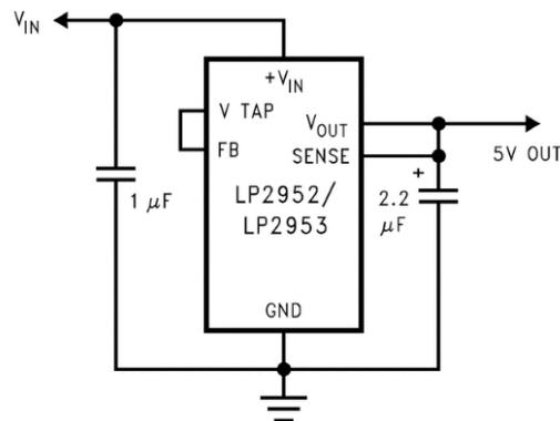
**Figure 3:** Linear Regulator LP2953 Schematic for 5V Fixed Output
