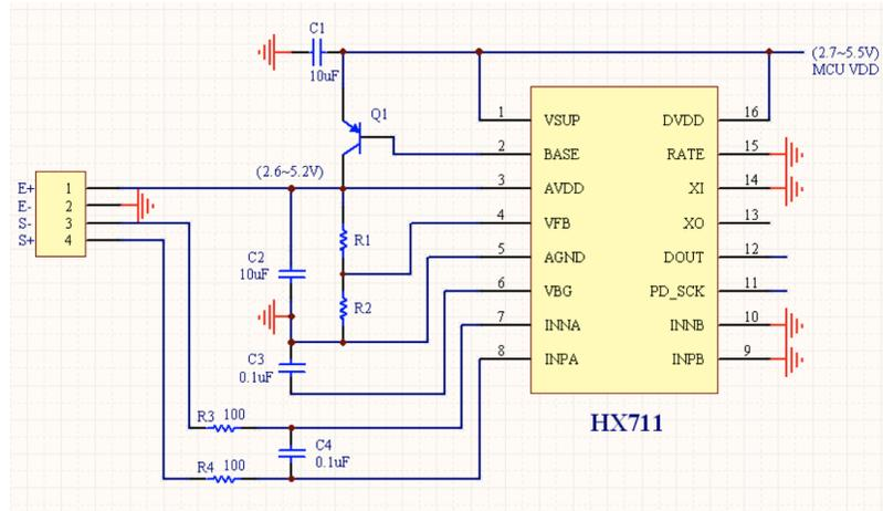
**Figure 4:** HX711 Module connected to Load Cell
