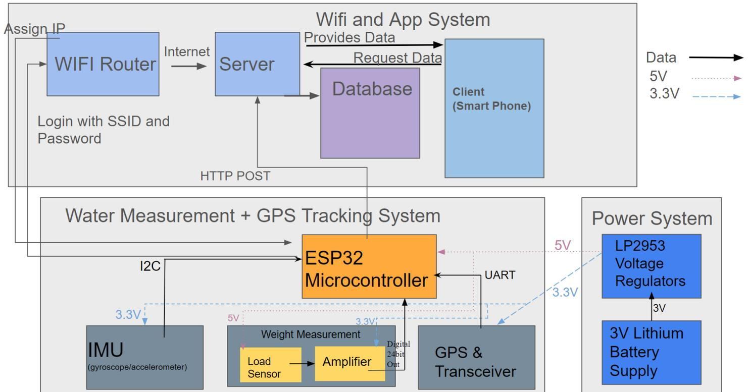
**Figure 1:** Block Diagram of Portable Water Tracking Attachment
