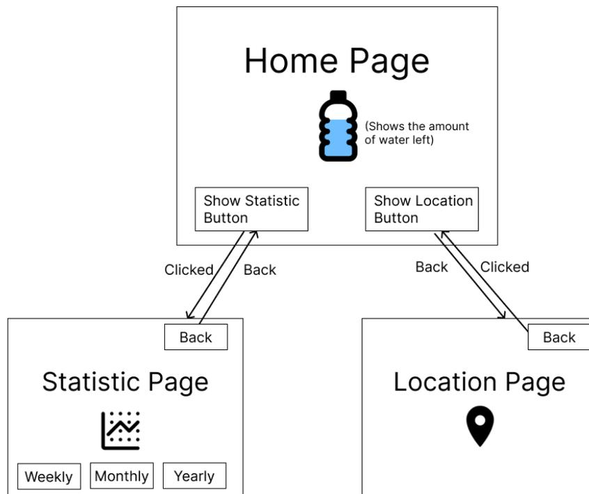
**Figure 12:** Front-End Application flowchart
