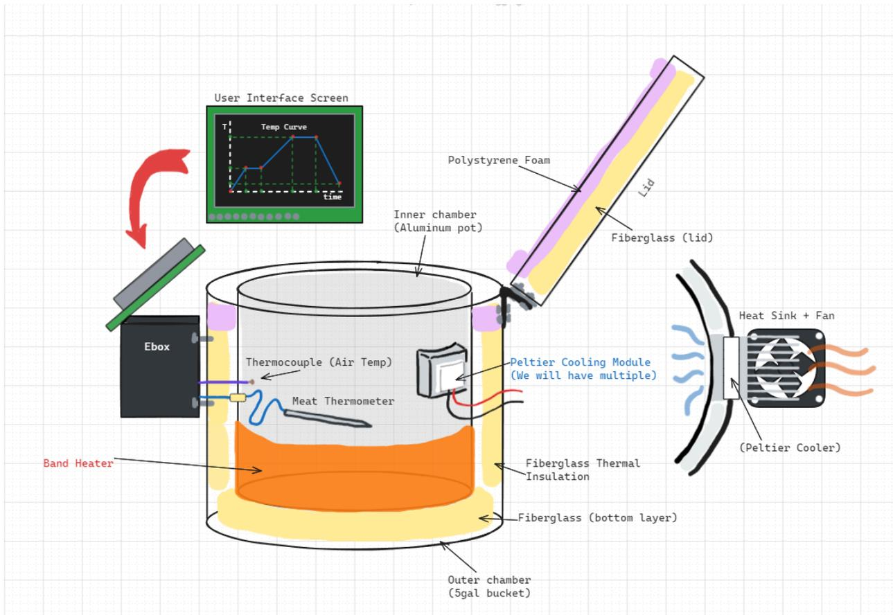
Figure 1: Temperature Controlled Chamber Design
