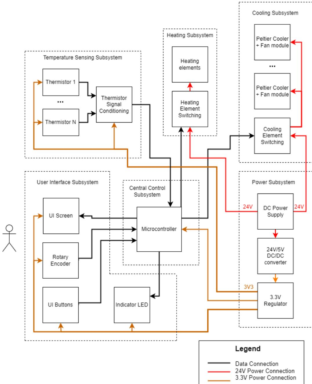
Figure 2: Block Design Diagram
