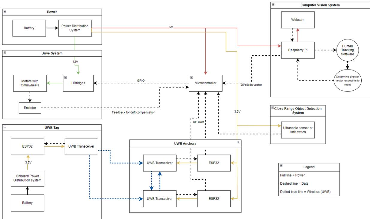
Fig. 2: High-level block diagram for our project.
