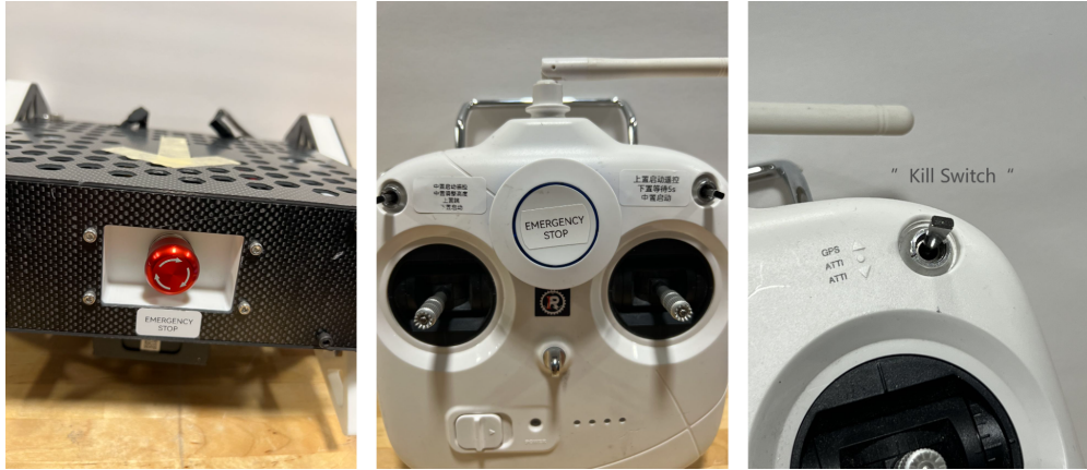
Figure 9: Emergency Stop mechanisms
