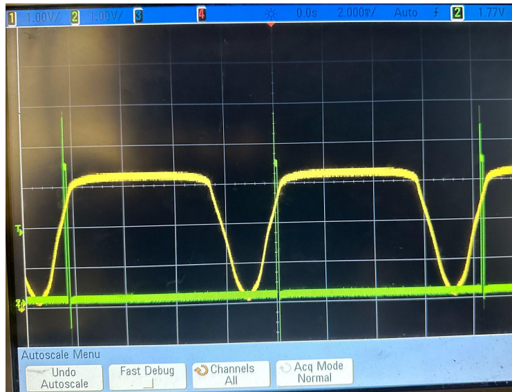
Figure 10: Oscilloscope reading showing pulse generated shortly after zero-crossing (bright bulb)
