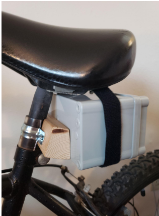
Figure 2.1.3.2: Indication Unit Enclosure Attached Under the Seat
