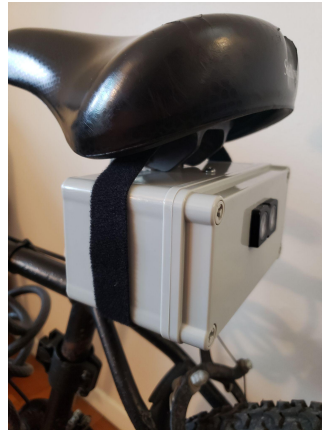
Figure 2.1.3.2: Indication Unit Enclosure Attached Under the Seat
