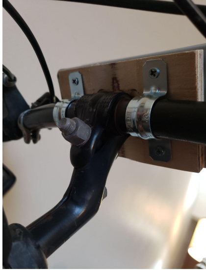
Figure 2.1.3.1: Indication Unit Enclosure Attached to Handlebar
