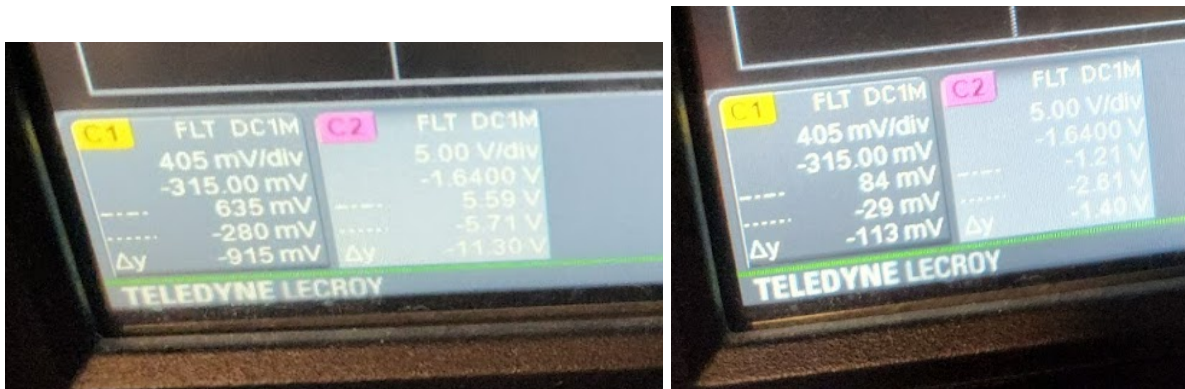
Figure 3.6: Peak-to-Peak voltage values of the input and output wave used for calculating gain.
