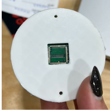
Figure 5: Enclosure Lid Exposing Image Sensor
