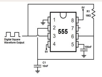
To create a 6Hz signal, R1= 10M $\Omega$  and C= 10nF. To create a 600Hz signal, R1= 100K $\Omega$  and C= 10nF. To create a 134Hz signal, R1= 470K $\Omega$  and C= 10nF. To create a 1.7KHz signal, R1= 33K $\Omega$  and C= 10nF. To create a 43KHz signal, R1= 1K $\Omega$  and C= 10nF. To create a 180KHz signal, R1= 150 $\Omega$  and C= 10nF. To create a 252KHz signal, R1= 100 $\Omega$  and C= 10nF.
