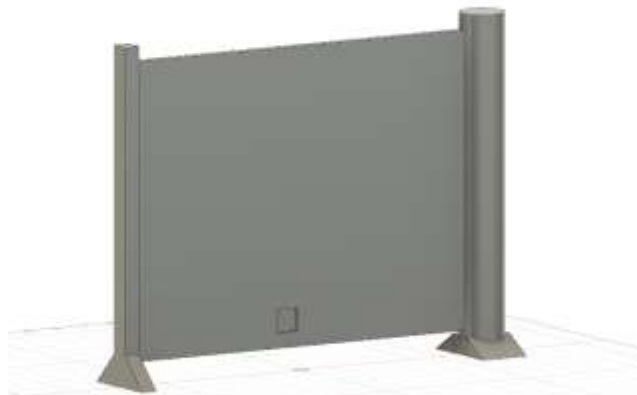
Figure 2: Front-side with sensor placement of the 18-inch wide gate
