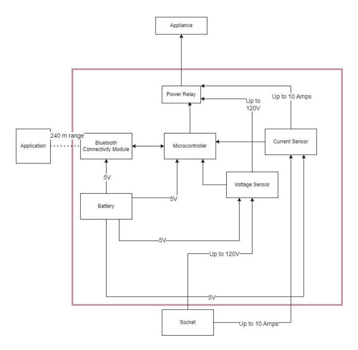
Our device is completely enclosed in the red box in the above figure. As shown in the block diagram, the device will be connected to the socket, the application, and the appliance. The current drawn from the device is measured and sent to the microcontroller and transmitted via the bluetooth module to the backend of our application.
