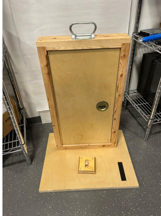
Figure 3: Our physical door and lock mechanism
