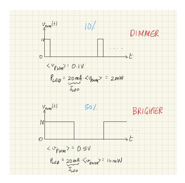
As seen above, this way the power to the LED can be adjusted and as along as the microcontroller can produce the PWM, the design will be successful. The microcontroller that we chose has two 8-bit timers and one 16-bit timer that can produce the PWM waveform.
